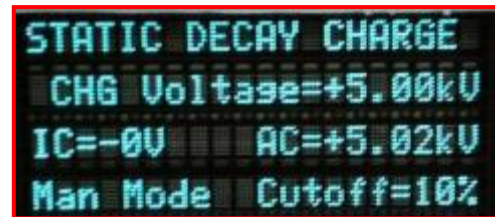
Figure 6-4: Sample with no IC and able to conduct charge
